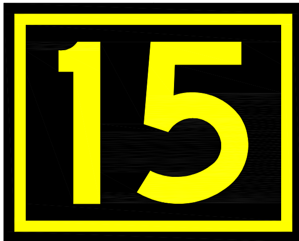
(b) Runway Location Sign
